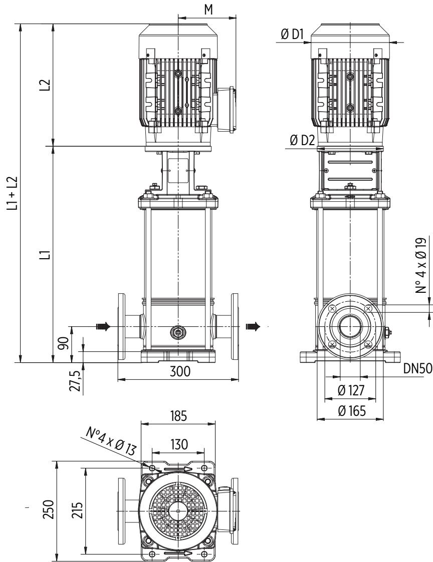
Round flanges on body type PN25/40: the pump is supplied without counterflanges (optional accessories, including bolts and joints)
