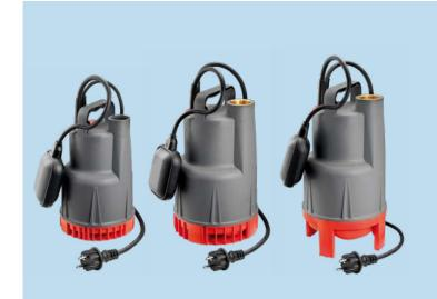
Drainage pumps for emptying pits and cisterns, for gardening; completely constructed in anticorrosive material. Brass insert on the delivery opening (DP 80/100 - DPV 80/100). The single-phase version includes a built-in capacitor, a thermal protector and it can be equipped with a float switch.
