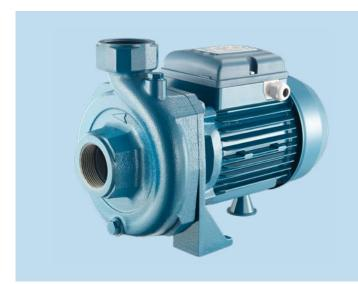
Medium delivery centrifugal pumps for agricultural applications. Equipped with an open impeller that allows the pumping of nonclean liquids, guaranteeing the free passage of small solids (Ø max. 10 mm).
